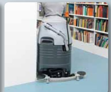
The new squeegee does not swing, (it moves only when hitting obstacles) so it perfectly follows the deck/water track and guarantees a complete water pick-up, even on tight turns, without leaving any trace
