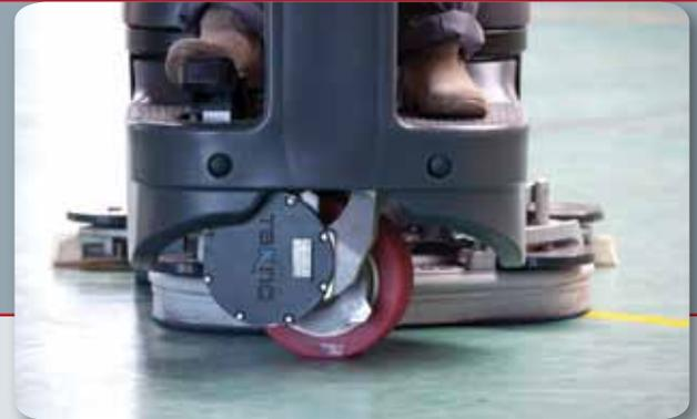
New deck system (linked to the steering wheel): when turning the steering wheel on the left, deck is moving on the left as well (same on the opposite side); it guarantees the best cleaning performance with maximum comfort and minimum effort. The water track is completely covered by the squeegee and side skirts are no longer required
