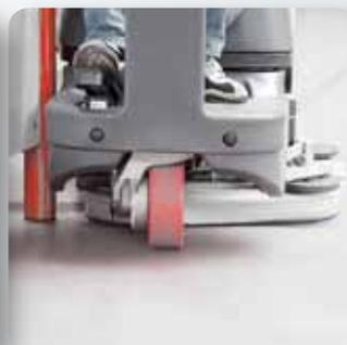
Deck is protected, by big bumpers and moves inside the machine body if hitting an obstacle (machine and environment protection)
