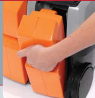
Batteries are easily accessed for charging and replacement. Orange batteries for warning/safety.
