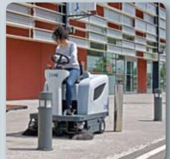
The SR 1101 is designed to handle both big and small cleaning situations, and can manoeuvre in tight spaces or climb ramps with as much as a 20% incline
