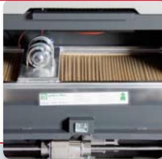
An electrical filter shaking systems cleans the filter automatically every 5 minutes
