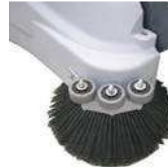
Side brush non marking roller bumper
