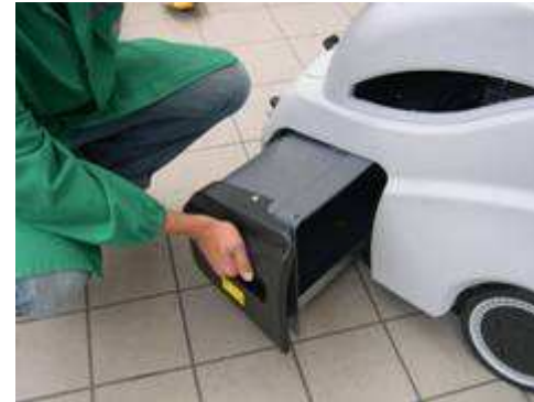
Light weight hopper material to allow easy discharge
