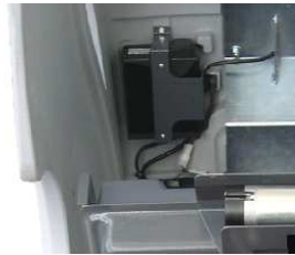
On board charger
