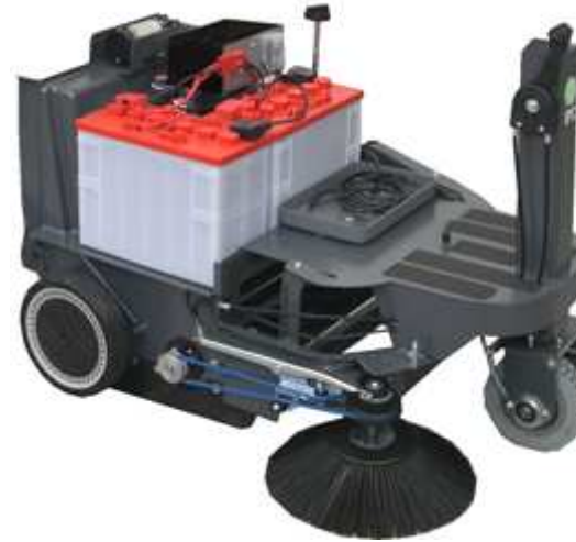
Fully coated steel frame structure
